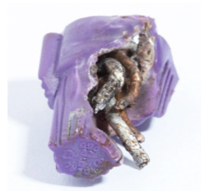
Wire Connector Designed for Copper Wiring Only
